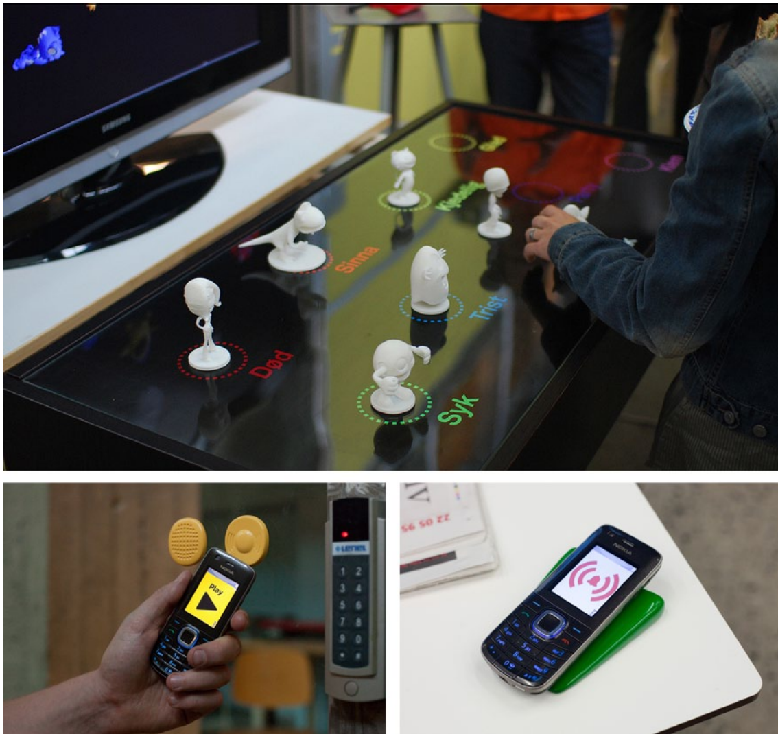
Figure 3. Three functional prototypes: (Top) The Orooni table, (lower right) the NFC alarm clock, and (lower left) the NFC office answer machine.
