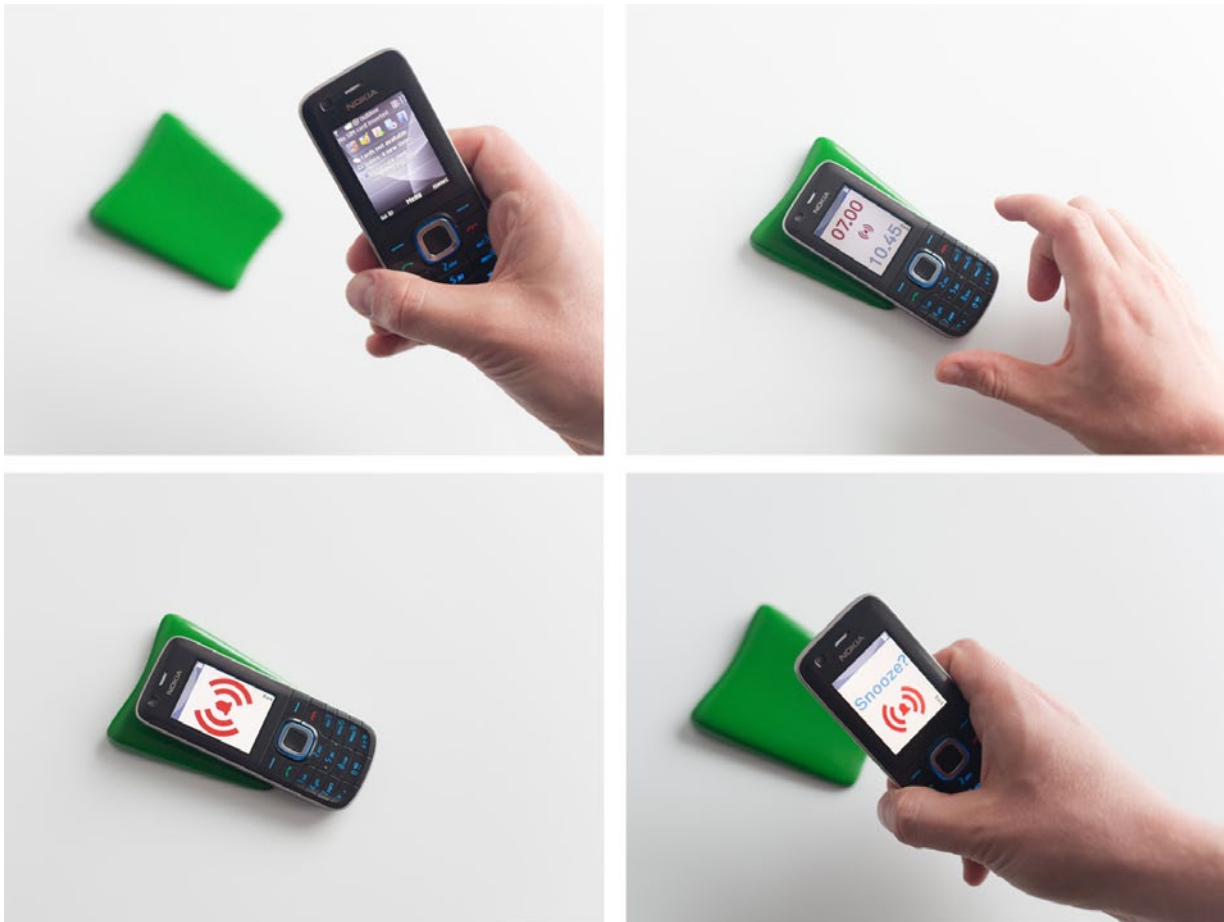
Figure 5. Tap and Hold gesture - NFC alarm clock using Tap and Hold interaction: (Top left) Phone is outside field. (Top right) The alarm is set and active while the phone rests on the tag. (Bottom left) The alarm rings while on the tag. (Bottom right) The alarm is stopped by removing the phone and the phone offers to start the snooze mode by putting the phone back on the tag.
