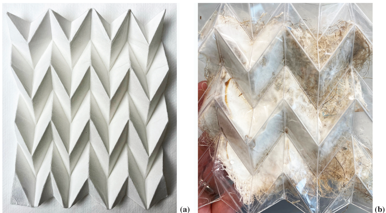
Figure 6. Miura examples: (a) structure folded from paper; (b) Reishi growth on fiber substrate.
