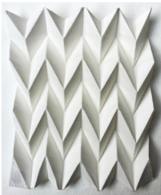
Figure 6. Miura examples: (a) structure folded from paper; (b) Reishi growth on fiber substrate.
