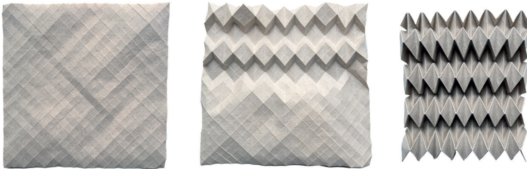
Figure 2. Folding an origami tessellation (from left to right): creating a grid, pre-creasing the unit cells, and collapsing the form into a dynamic structure.
