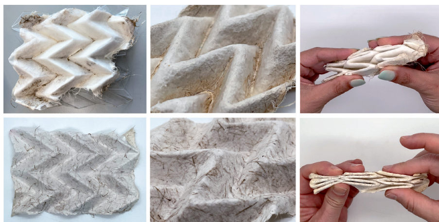
Figure 10. Grown tessellations: artifacts with mycelium/hemp (top row) and mycelium/pine (bottom row).
