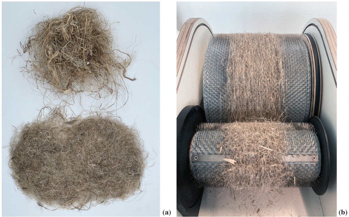
Figure A7. Carding hemp: (a) raw hemp pictured above carded fibers; (b) the mechanical carding process.
