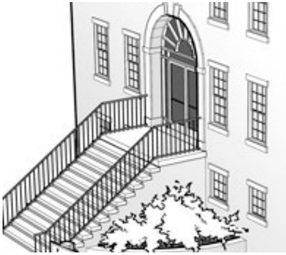
Figure 7. An inaccessible building entrance based on a stair morphology.
