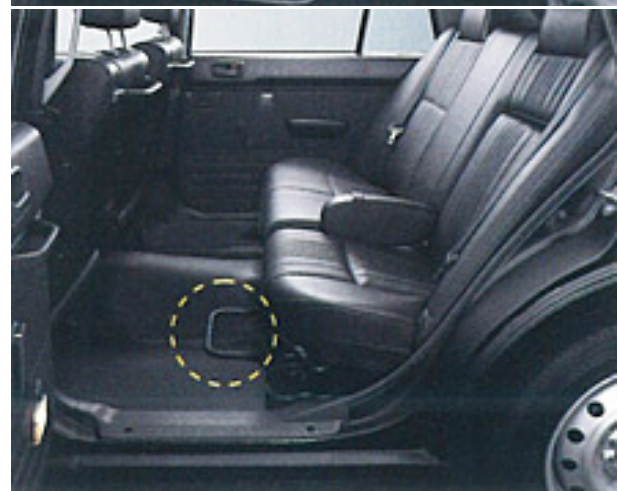
Figure 2. A UD rear seat design in a Toyota Crown Comfort (Toyota, 2009).
