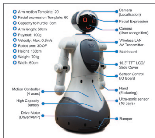
Figure 1. The specifications for Tiro's hardware and software.
