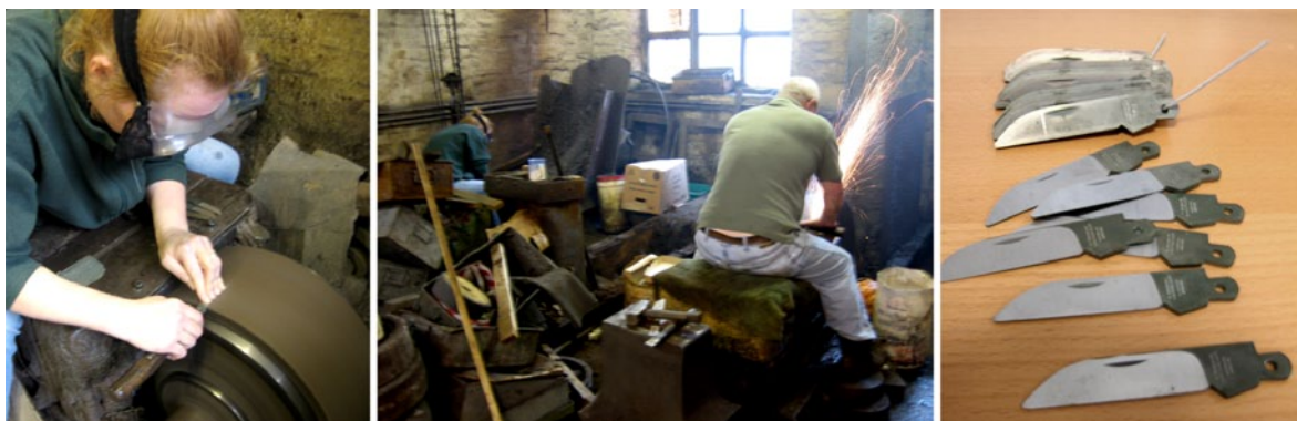
Figure 1 (left to right): Expert learner grinding, the craftsman’s workshop, blades from the manufacturer at the rear, and ground blades at the front.
