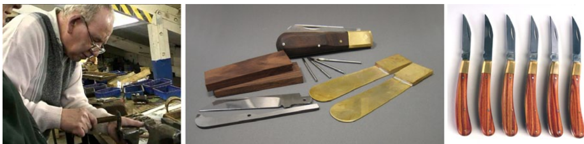
Figure 2 (left to right): The craftsman, parts of a traditional folding knife, set of "Etrick" folding knives made by the expert learner under the craftsman's guidance.
