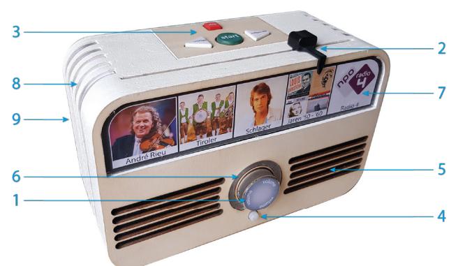
Figure 3. High-fidelity prototype of the music player, with the following components: 1. Volume knob, 2. Presets slider, 3. Control buttons (start, stop, previous, next), 4. Motion sensor, 5. Speakers, 6. Volume indicator, 7. Presets, images with light, 8. Product light, 9. Ambient light (on the back).
