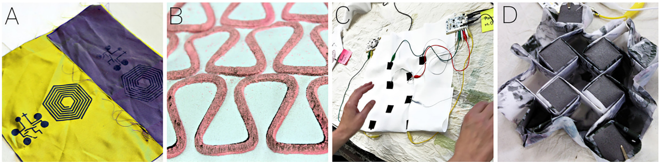
Figure 2. Soft Systems printed electronics workshop in collaboration with DZP Technologies held at the Royal College of Art: (a) capacitive sensor screen-printed on silk substrate by Jonna Saarinen; (b) capacitive sensor with puff-binder overlay by Emma Harriet White; (c) testing by Jonna Saarinen; and (d) pleated switch by Tsai Chun Huang and Amy Winters.
