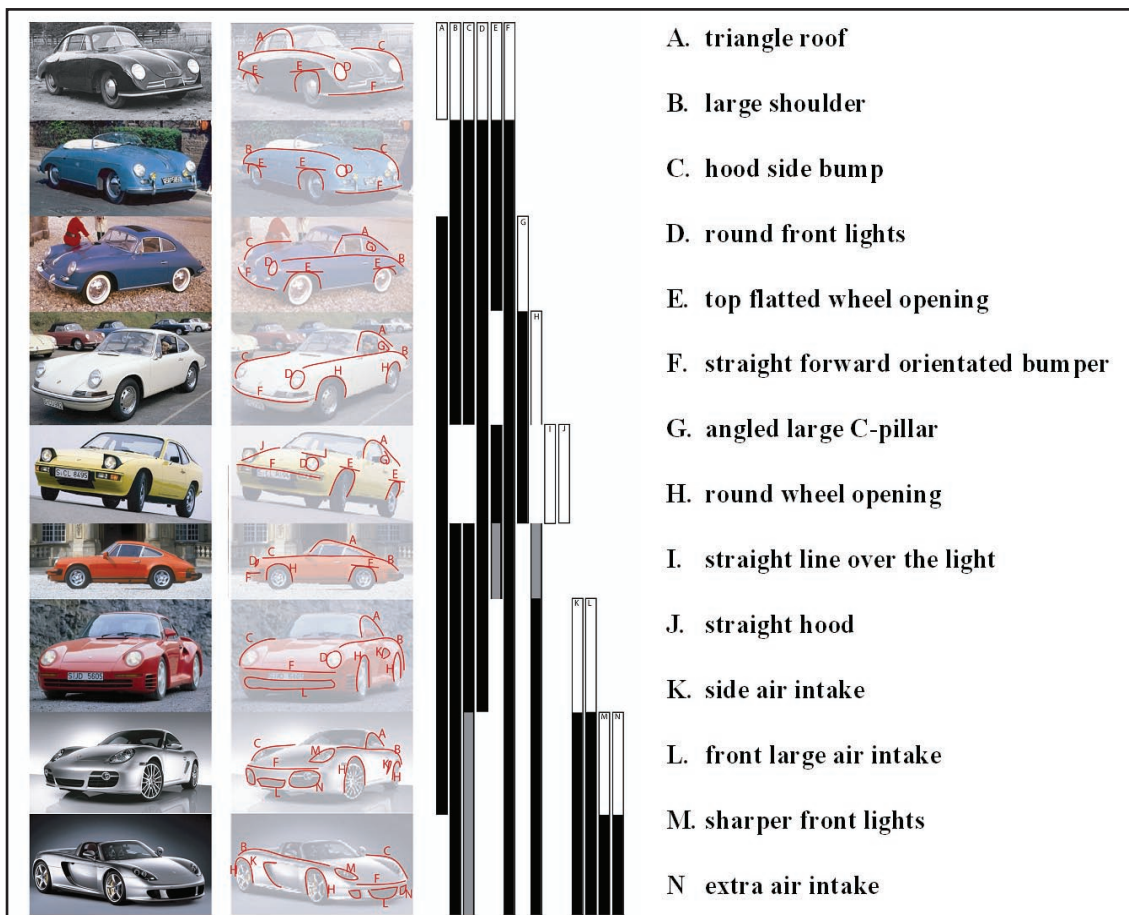
Figure 8. Design history analysis of Porsche performed by Group 8/2005 (Niklas Fahlquist and Fernando Pizer).
