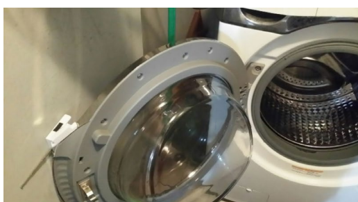
Figure 14. The door contact sensor attached to the wall and the washing machine door from H2 (left). Two hours after starting the washing machine, H2_M and H2_F received the text message (right).
