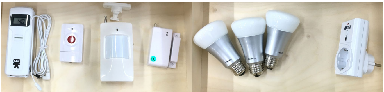
Figure 11. Sensors and actuators in Routinoscope (from left): temperature-humidity sensor, wireless switch, motion sensor, door contact sensor, smart light bulbs, wireless socket.
