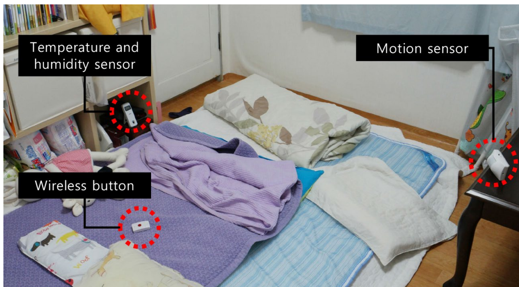
Figure 13. Motion sensor, wireless switch, and humidity/temperature sensor in the new baby room (H2; from H2_M diary).
