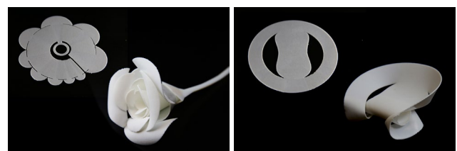
Figure 3. Programmable and 4D printed self-folding rose (left) and chair (right), triggered by heat, by Morphing Matter Lab, Carnegie Mellon University.
