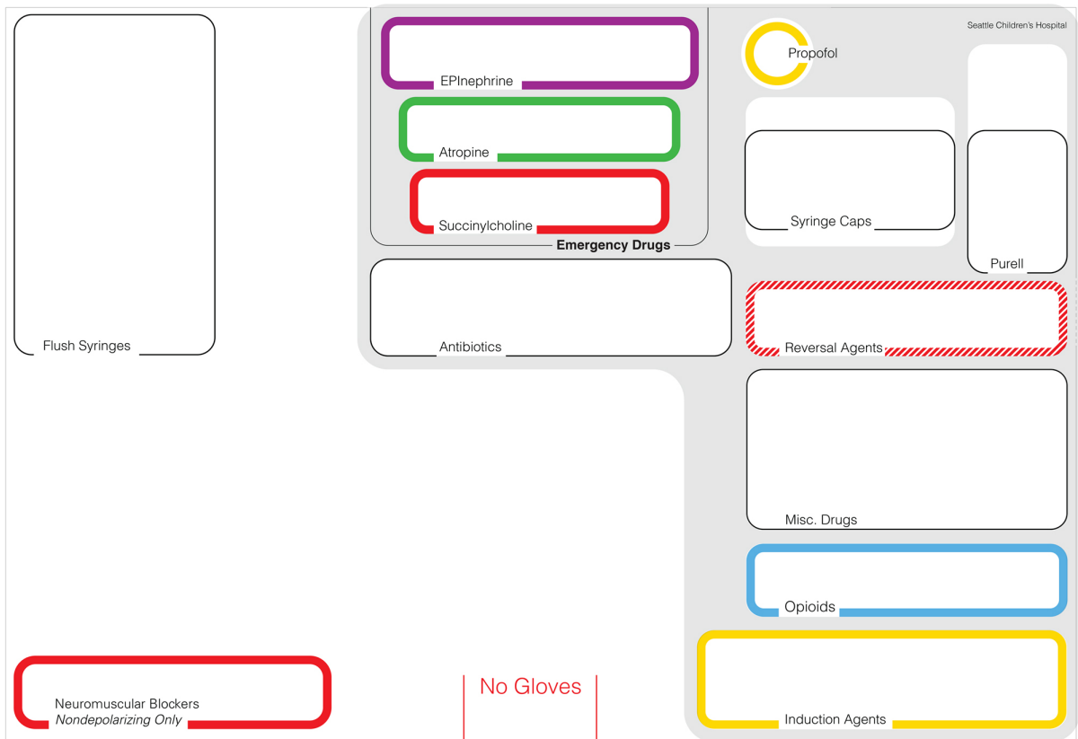
Figure 7. Laser cut transparent acrylic overlay to prevent medications from shifting locations when the anesthesia cart is moved.
