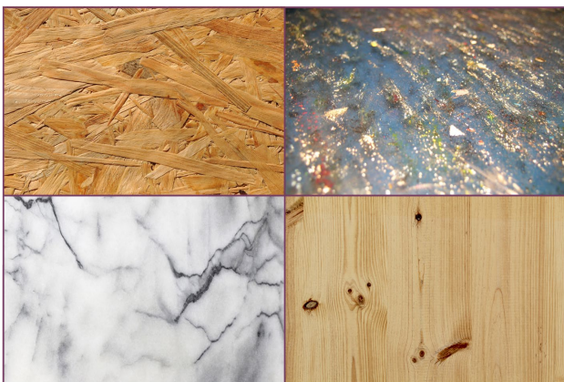
Figure 2. Material surface imperfections inherent to synthetic and natural material surfaces. Clockwise from top left: chipboard (© Petr Cihak | Dreamstime.com), recycled polycarbonate from discarded compact discs, pine (© Jordi Clave Garsot | Dreamstime.com), marble (© Siloto | Dreamstime.com).
