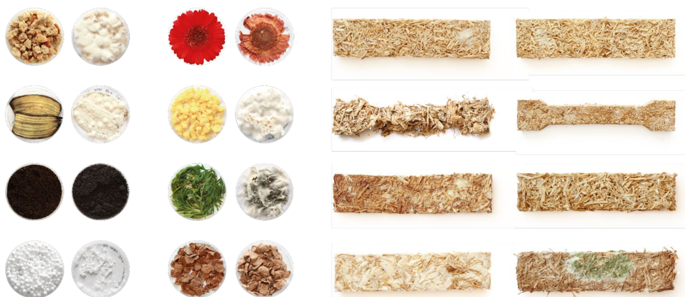
Figure 7. Initial tinkering with the material by trying different substrates such as bread particles and orange peel (left); second round of tinkering with the material with sawdust as substrate (right).
