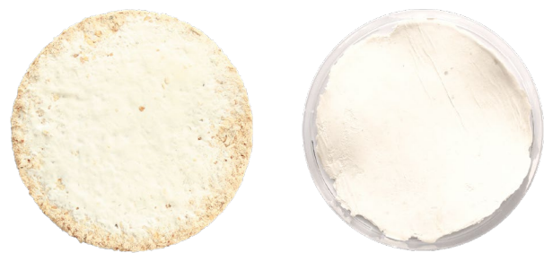
Figure 2. Mycelium-Based Composite (left) and Pure Mycelium (right).
