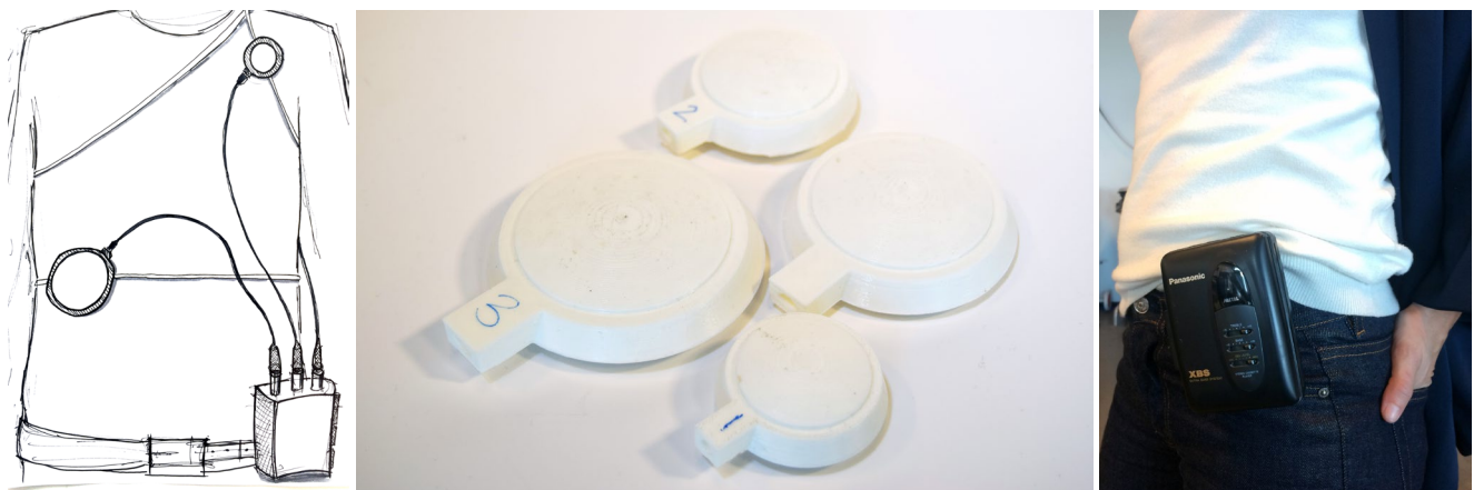
Figure 13. Left: A concept sketch of the Hedonic Haptic player. Middle: rapid prototypes of different sized domes for the vibration motors. Right: the look and feel of a Walkman.
