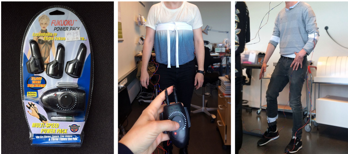
Figure 8. Getting familiar with vibrotactile stimuli. Left: an off-the-shelf vibration motor kit. Middle and right: vibration motors sewn in fabric bands and strapped on the body, with the remote to control the intensity of the vibrations.
