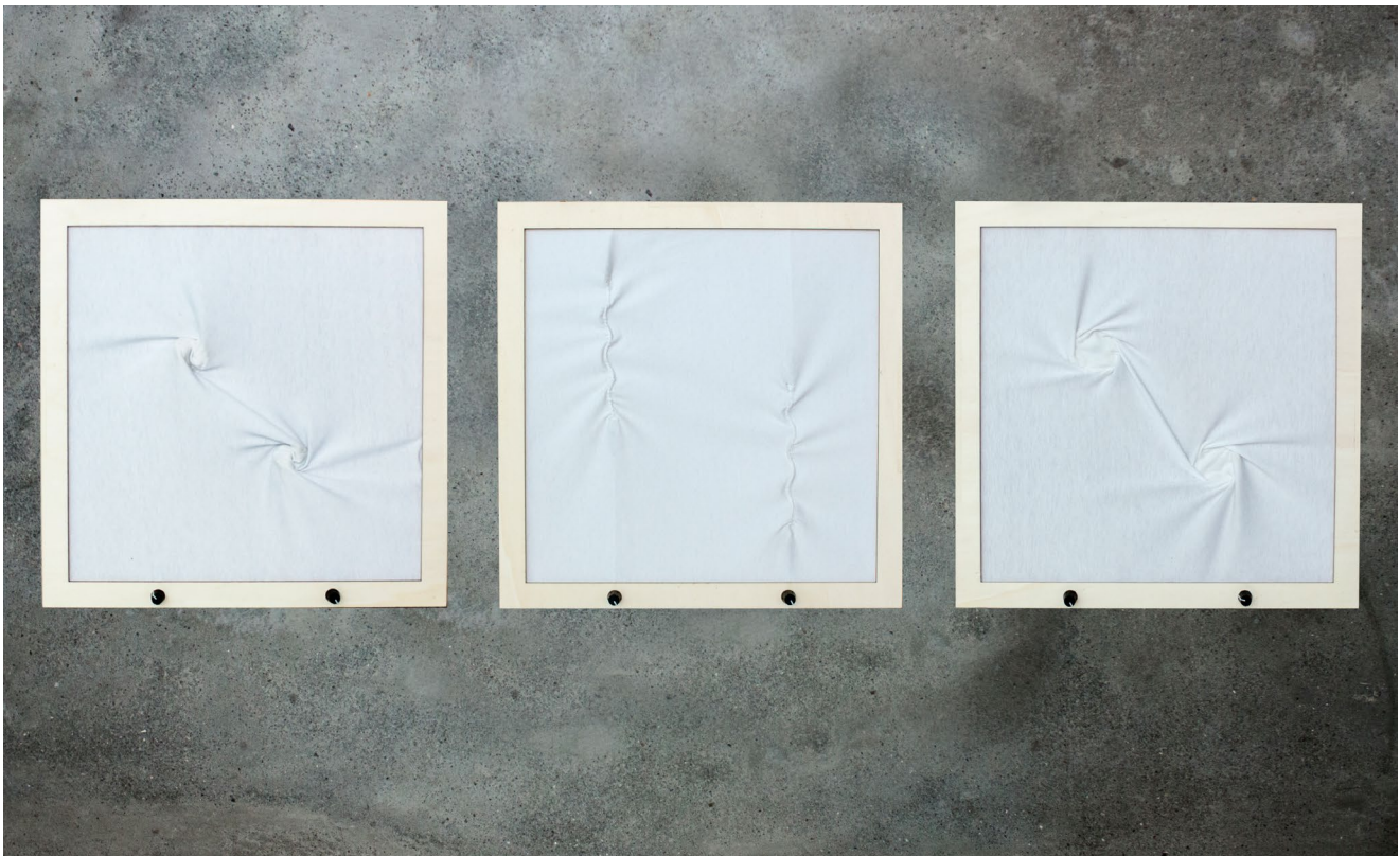
Figure 1. The three boxes, the left-hand one powered by two stepper motors, the middle one by two helical strings of shape-memory alloy, and the right-hand one by two servomotors. All three boxes are 20 inches in length and width and four inches high. See also the temporal forms in action at https://vimeo.com/album/3639572 .
