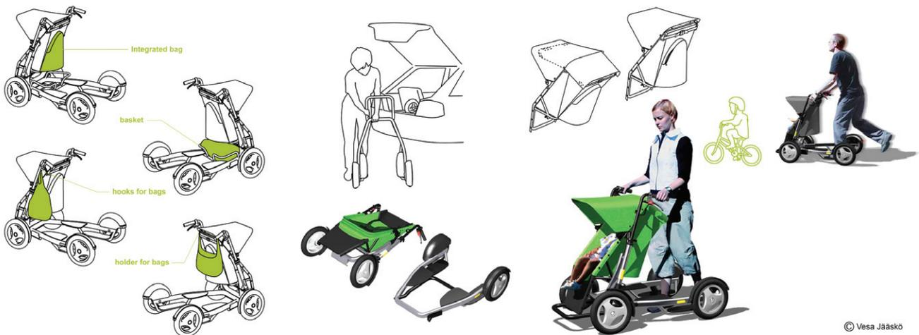
**Figure 7: Illustrations and renderings generated for the concept presentation.** The figures show alternative solutions of carrying different loads, adjustable seat feature, collapsible structure option, and scenarios of traveling with children of different ages. Drawings and renderings by Vesa Jääskö.
