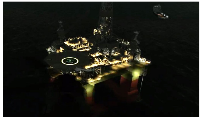
Figure 7. Frame from a simulation of a helicopter approaching a rig helideck at night. The LysTech light system is shown by the yellow circle and green "H".
