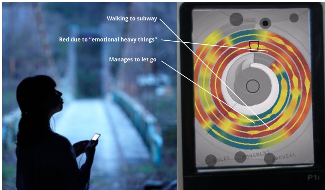
Figure 1. Affective Health interface: The continuous measurements of skin conductance, pulse and movement are presented in a spiral form with the most recent data in the middle and history spiralling outwards. The resulting visual representation is legible to the user in the sense of recalling specific situations and forming the basis for interpretations.
