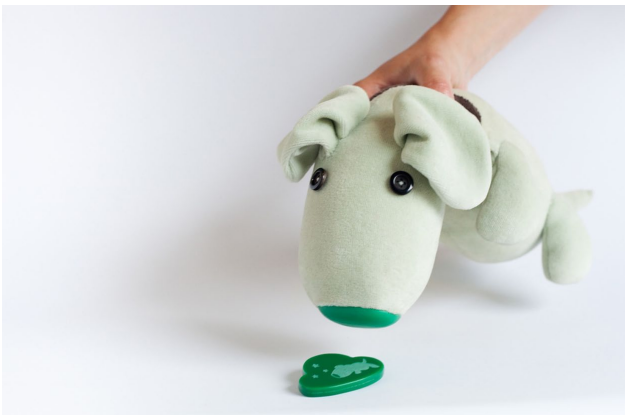
Figure 5. The toy dog 'Sniff'. Sniff has an RFID reader in his nose, and when he encounters RFID tagged objects, various sounds and haptic feedback are triggered.
