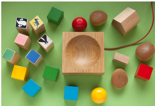
Figure 6. An image of the 'Skål' or 'Bowl' prototype. A wooden bowl contains an RFID reader and sits in the middle of a number of a number of smaller objects that contain RFID tags. When these objects are placed in the bowl they trigger media playback on a connected television.
