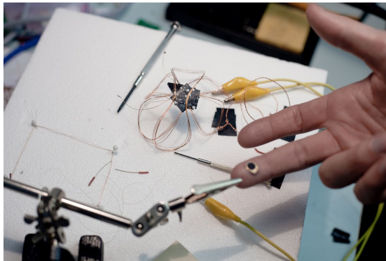
Figure 2. Exploring the technical material of RFID: an RFID tag is being taken apart on this workbench in our design studio. The looped wire antenna as well as the tiny memory chip resting on the finger are shown.
