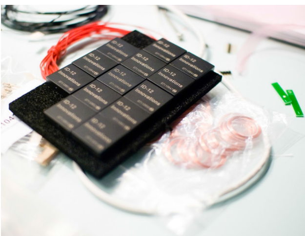
Figure 7. A package of 'Innovations ID-12' RFID modules as they arrive from the manufacturer.
