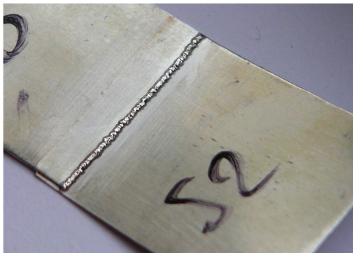
Example 1: welding two sheets over edge
