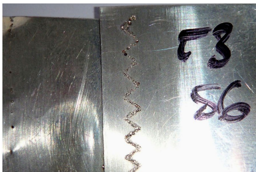
Example 2b: Welding two sheets flat (zigzag)
