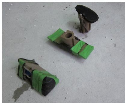
**Figure 12. Group 2's prototypes:** The first two prototypes to the left were inspired by boats; the foot should cut through water just like the hull of a boat. The third prototype was intended to function as a stilt when attached to the bottom of the prosthetic foot. The group believed that the narrow shape would prevent it from getting stuck in mud but emphasized that this solution would only be useful when walking in shallow mud.
