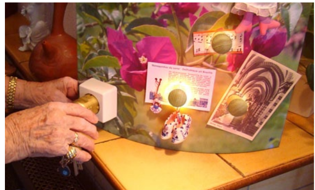
Figure 2. The KeyPing prototype consists of a board with keys and personalized tokens.
