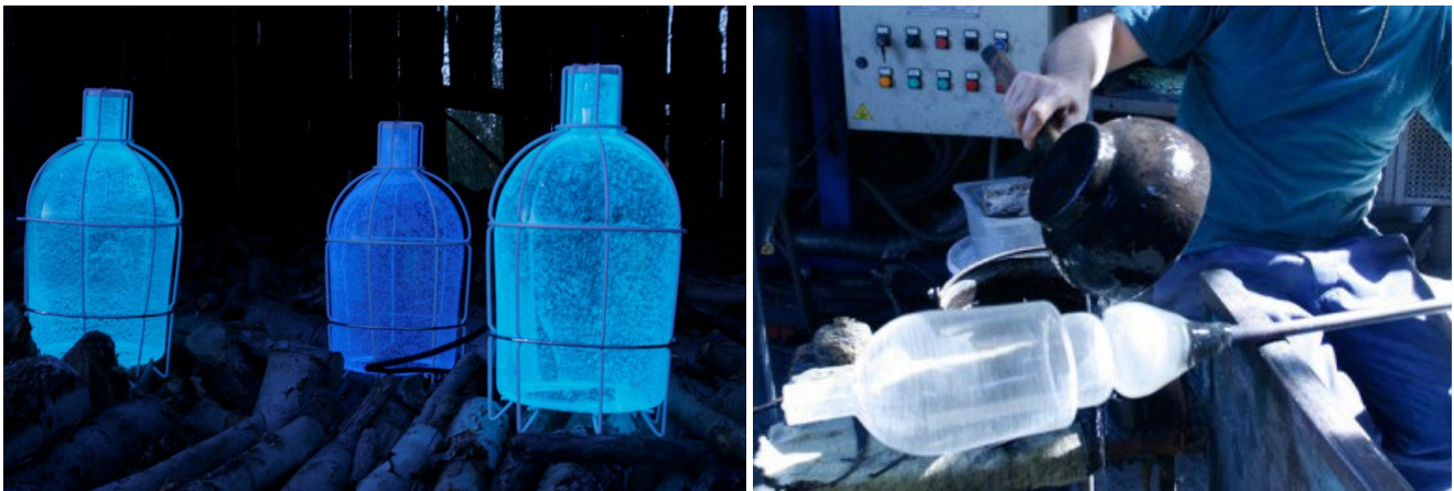
Figure 11. Designers exploit the potential for embedding photoluminescent pigments into the transparent body of glass, using a traditional technique: left, Trap Light by Gionata Gatto and Mike Thompson; right, Murano glass blowing process (image source: Studio Gionata Gatto; reprinted with permission).
