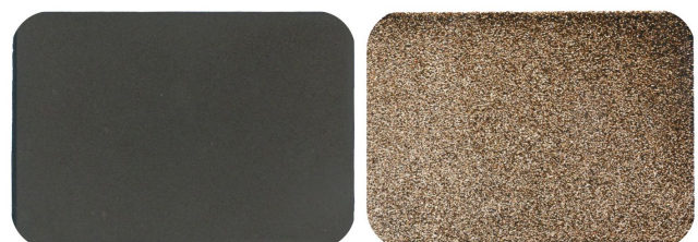
Figure 2. HIPS resin Satin finish 16.53 and ABS resin Satin finish 46.14 used as evaluation samples.
