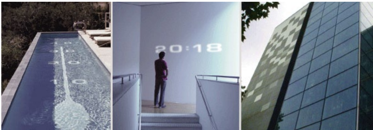
Figure 2. Chronos Chromos Concrete can change color in response to a computer's output. The composite is made from thermo chromatic ink, nickel chromium wire, computers, and concrete (Ritter, 2007).
