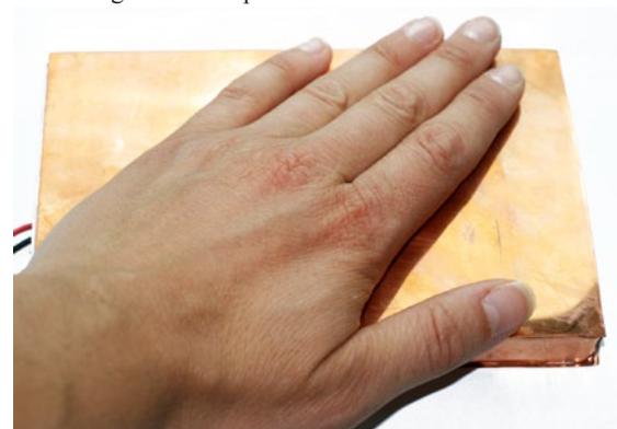
Figure 11. By placing a hand on top of the tile one senses the tiles reaction to the heat form the hand as it after a short period turns cold.
