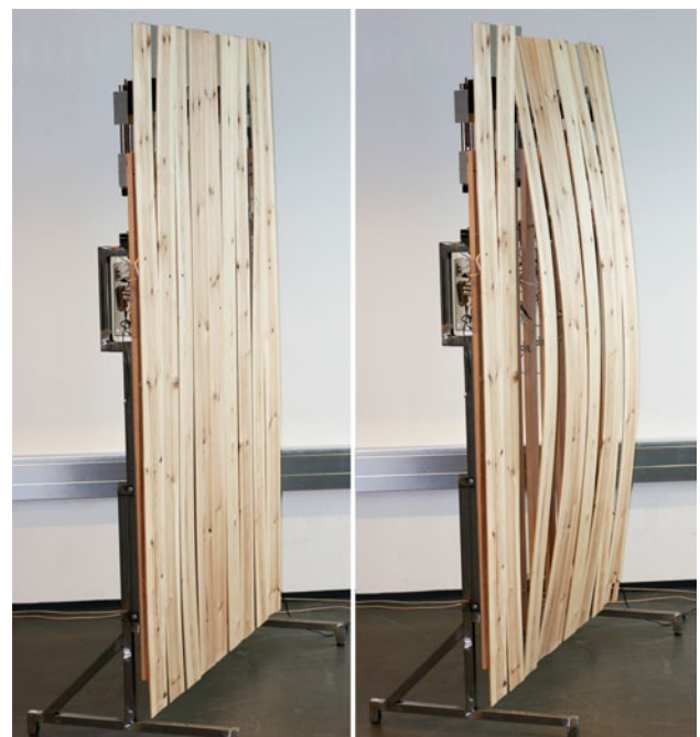
Figure 3. PLANKS: planks of pinewood flex as a reaction to sonic activity in their vicinity. Each plank works individually and can be used for a variety of different purposes such as wall panels or doors. The composite is made from pine planks, motors, microphones, and an Arduino computer (Vallgård, 2008).
