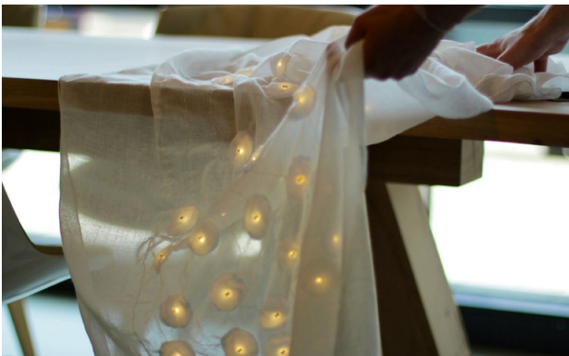
Figure 2. Soft Interiors (Kassenaar, 2011): A semi-transparent woven fabric with laminated LED lights and inductive charging.
