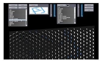
Figure 7. The Pixel Tool allows designers to adjust a range of parameters for simulating content on the pavilion façade.
